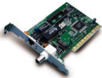
A network card that uses a standard cable network socket.
