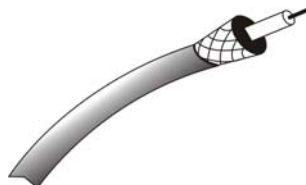
Figure: Coaxial Cable
